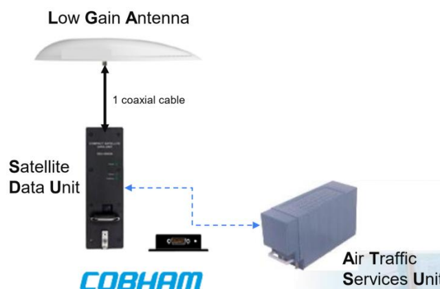
Figure 5-1: FANS-C over SatCom Avionics
