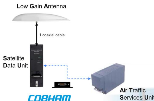
Figure 5-1: FANS-C over SatCom Avionics
